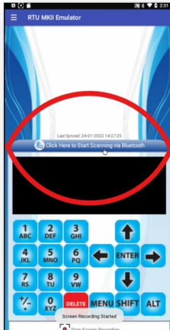
Step 3. A “Bluetooth Discovery” screen will appear and automatically start scanning for any PA Bluetooth Dongle that is available.
