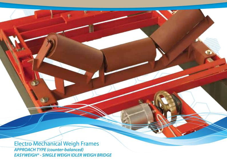
This model incorporates a low deflection, rugged *counter-balanced*, single weigh idler, approach type weigh bridge with a single, precision load cell, operating in tension. The *load sensor assembly incorporates overload protection* and protection against mechanical shock.
