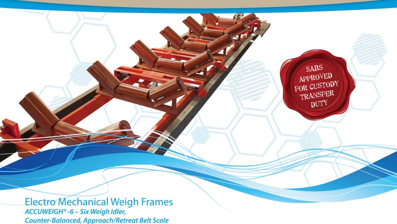
This model incorporates a low deflection, rugged, counter-balanced, six weigh idler, Approach/Retreat weigh bridge design with a single, precision load cell, operating in tension, to provide superior weighing performance over extended periods with minimum maintenance. The load sensor assembly incorporates overload protection and protection against mechanical shock.
